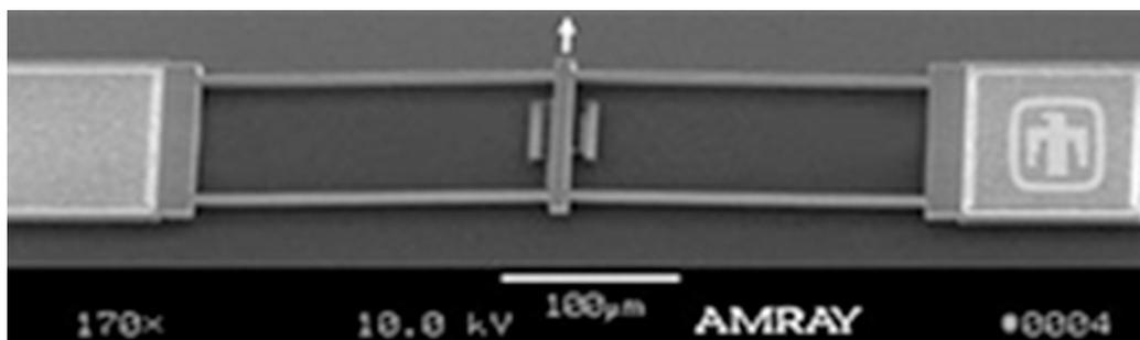
Figure 2. V-shaped thermal actuator. The constrained thermal expansion of the angled beams results in the motion of the centre shuttle in the direction indicated by the arrow. (Image courtesy of Sandia National Labs).
