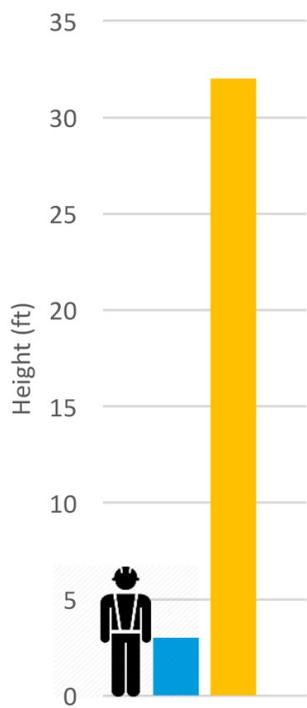
Figure 1. Blue – FAST tool; Yellow – typical array PLT string.
